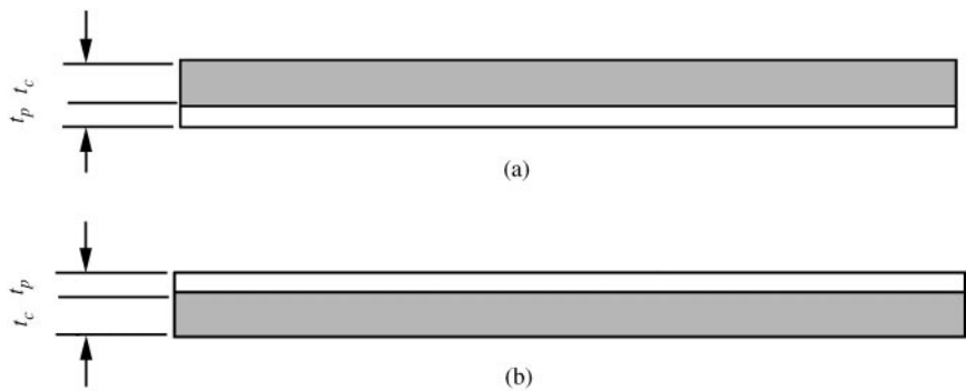
Figure 2. The geometric schematic of two-layer plates: (a) A plate with a coating layer above; (b) A plate with a coating layer below.
